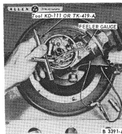
FIG. 11 Adjusting New Breaker Point Gap
